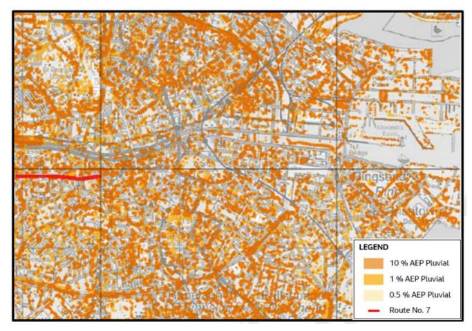
Figure 4.17 Extract of pluvial flood mapping on the Route No.7 bus corridor Kilmainham to City Centre
